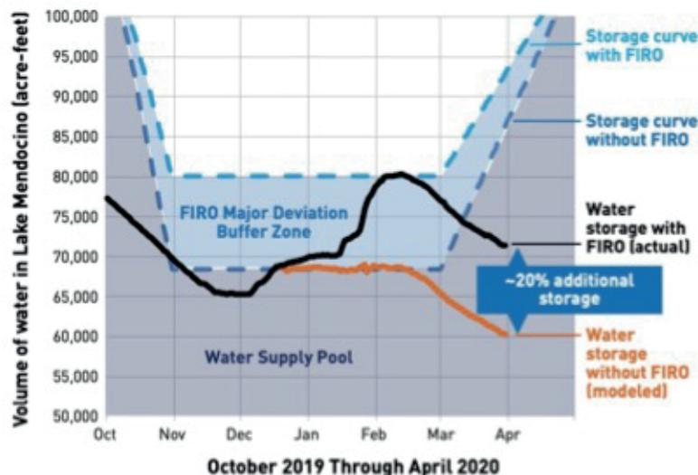
Figure 2. Lake Mendocino storage increased by about 20 percent during major deviation operations in WY 2020, compared with modeled storage without FIRO, during a year when precipitation was 38 percent of average.
